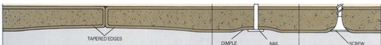
Figure 9.3 A plasterboard cross-section
